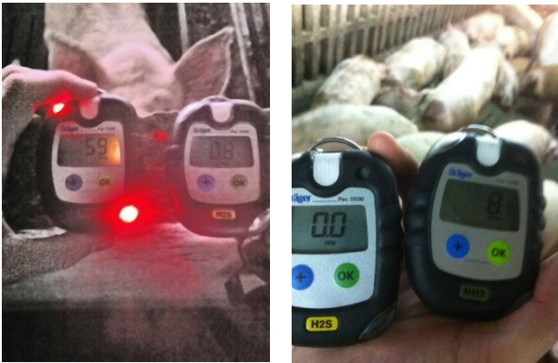
Control hall (left) and test hall (right) NH 3 and H 2 S monitoring.
